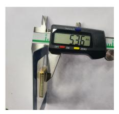
**Step 3.** (in package): Check Measurements Against. 17.8mmx30mmx5.3mm= **Gold Should Have**: 1,610 cubic mm per 1 troy ounce
